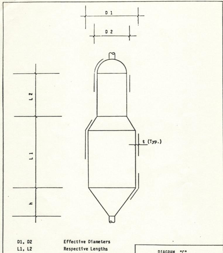
h t Height of Conical Head Insulation Thickness
