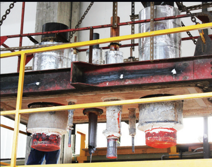
Floor post-test exposed and unexposed face
