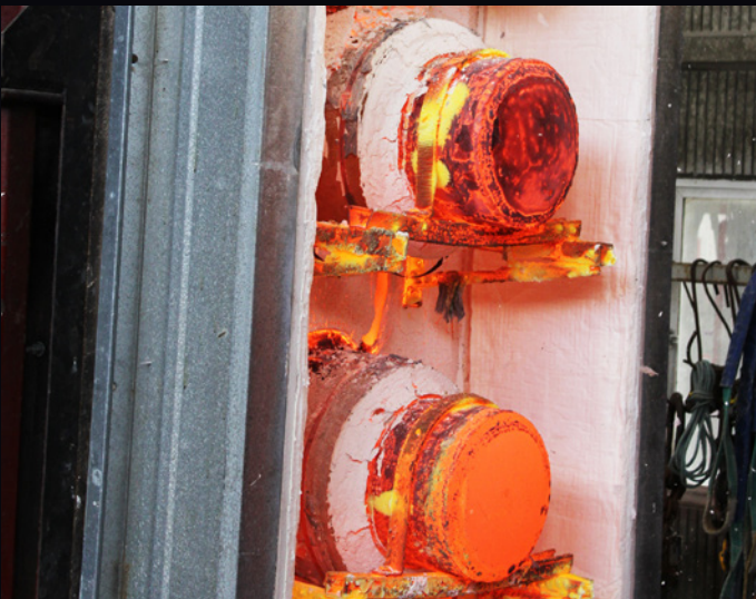
Wall post-test exposed face
