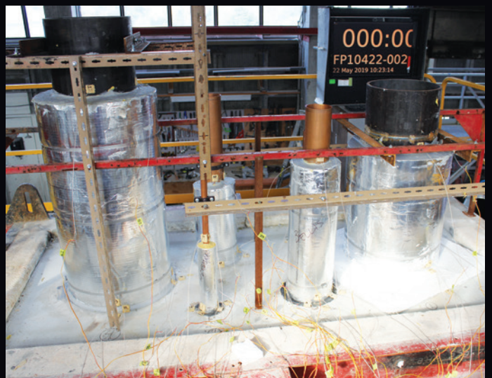
Floor pre-test unexposed face
