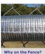
In our <u>December newsletter</u> we included this photograph of a length of insulation fixed to a chain link fence. It was fixed to the fence in September and has now been there for 6 months. It is of course a length of our Therm-o-lag chemically cross linked polyethylene spi, sealed along 50% of it's joint with PPC 493 tape x 50mm wide. The remaining joint is sealed with Venture 1529 HD x 50mm tape.
